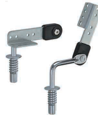
SSIC-RH-201 Material: Iron Finishing: Zinc plating Pitch:9°/Step Working Range: 90-162° /90-180°
