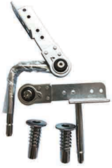
SSIC-RH-101 Material: Iron Finishing: Zinc plating Pitch:7.5°/Step Working Range: 90-135° /90-165°/90-180°
