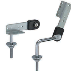
SSIC-RH-202 Material: Iron Finishing: Zinc plating Pitch:9°/Step Working Range: 90-162° /90-180°
