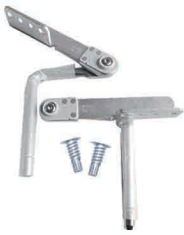
SSIC-RH-501 Material: Iron Finishing: Zinc plating Pitch:3°/Step Working Range: 90-135° /90-180°/90-210°
