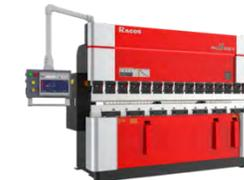
Single/Dual servo hybrid CNC Press Brake
